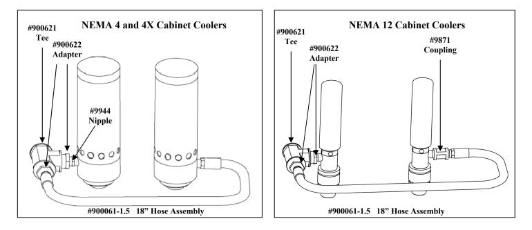
**For NEMA 4/4X Cabinet Coolers**, install the #9944 1/4 NPTM X 1/4 NPTM Nipple in the inlet of the first Cabinet Cooler. Use a #900622 1/2 NPTM X 1/4 NPTF Adapter to connect the #900621 Tee to the first Cabinet Cooler. Use the other #900622 1/2 NPTM X 1/4 NPTF Adapter to connect the #90061-1.5 18" Hose Assembly to the #900621 Tee. Connect the other end of the hose directly to the second Cabinet Cooler. The #9871 Coupling is used for NEMA 12 models and is not needed for this assembly.
